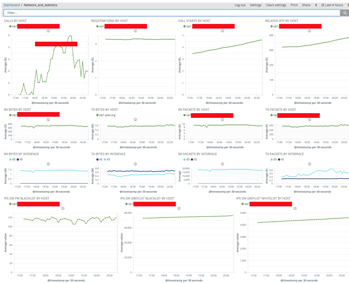
Fig. 40: Network Statistics Dashboard Capturing a Failover Situation
